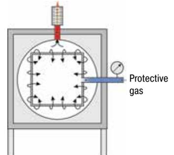
**Safety Concept for Heat Treatment under Flammable Process Gases**
