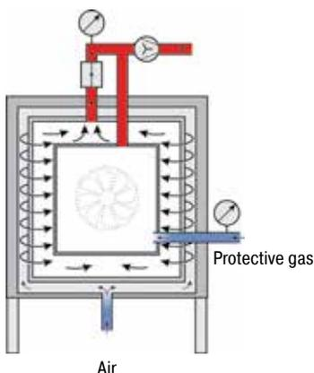
**IDB Safety Concept in Retort Furnaces for Debinding under Non-Flammable Protective Gases or for Pyrolysis Processes**
