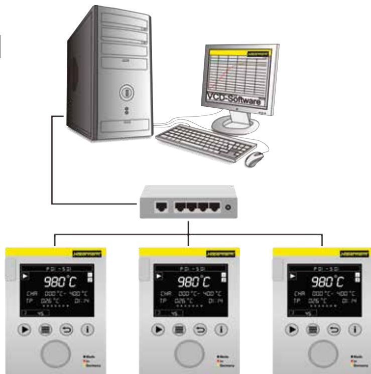
Example lay-out with 3 furnaces
