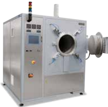
Hot-wall retort furnace to 1100 °C
