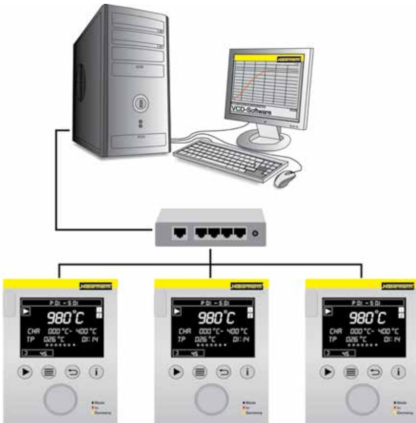
Example lay-out with 3 furnaces
